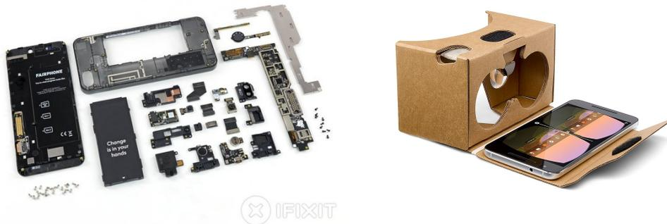
**Figure 1.** On the left, a picture of the Fairphone, a smartphone aiming to have a lower environmental footprint and better social impact than others in the market. In particular, its modular internal hardware focus on accessible and easy repairation. On the right, a cardboard virtual reality headset for a smartphone.
