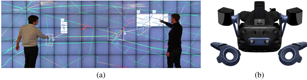
Figure 1. The intern will work with (a) the WILDER wall ( 6 \times 2 meters for 14\,400 \times 4\,800 pixels, driven by a rendering cluster of 10 workstations, and equipped with an air-gesture tracking system and a touch sensitive frame) and (b) two Vive Pro Head Mounted Displays.
